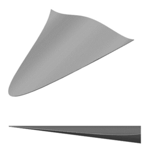
Figure 3: Waverider Geometry in Isometric View (top) and Side View (bottom)
